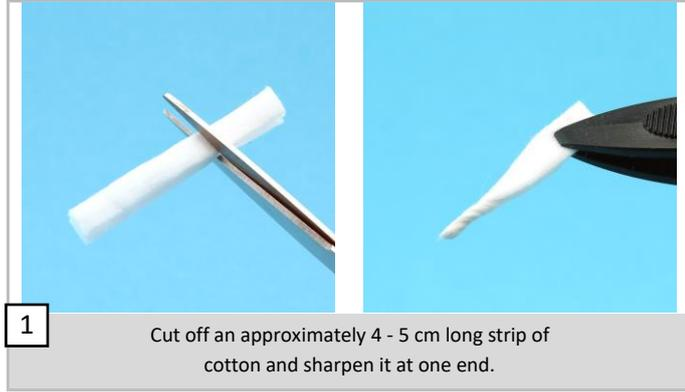
1 Cut off an approximately 4 - 5 cm long strip of cotton and sharpen it at one end.
