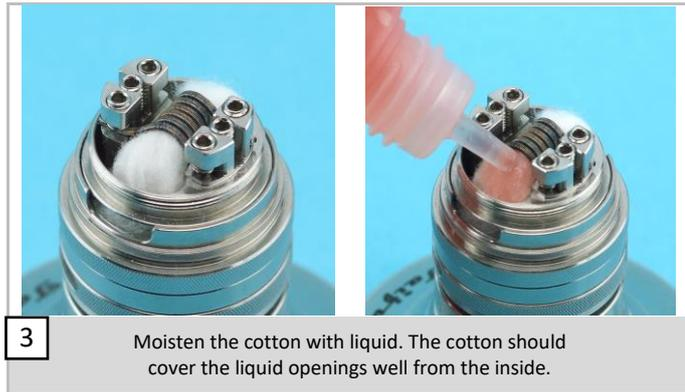
3 Moisten the cotton with liquid. The cotton should cover the liquid openings well from the inside.
