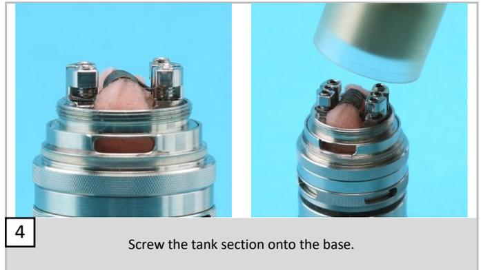
4 Screw the tank section onto the base.
